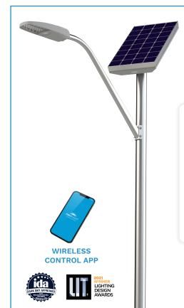
The BFL Series solar LED street light is a great fit for residential and collector street lighting as well as parking lot lighting applications. The self-contained, unobtrusive solar engine design integrates its solar power, battery and adaptive control capabilities into a compact and simple form. This, combined with an efficient LED fixture, makes the BFL Series an excellent fit where high performance, full cutoff and cost-effective lighting is required.
