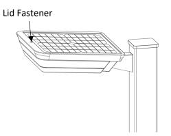
**7. REMOVE PACKAGING AND CONNECT BATTERY CABLES.** Remove packaging material from interior of light and connect the battery cables, **ensuring to latch the connectors.**
