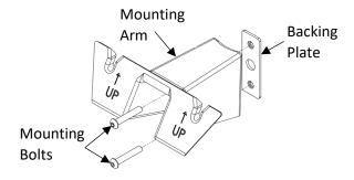
**4. ATTACH MOUNT TO POLE.** Insert backing plate into pole and thread bolts fully into backing plate through the mounting arm. Ensure flat side is placed against the inner surface of the pole. Torque bolts to 70 inlbs.
