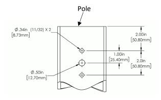
**2. REMOVE MOUNTING BOLTS FROM MOUNTING ARM.** Remove mounting bolts using 5/32" hex key.
