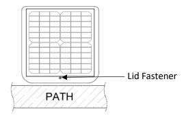
**3. TIGHTEN SCREWS.** Tighten 4 setscrews with 1/8" hex to snug (65 in-lb if using a torque wrench).
