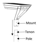
**2. ORIENT TO PATH.** Orient the light with respect to the path as shown.
