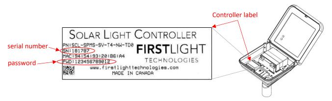
For this solar light to work properly, you **MUST** set the light's clock at the time of install. This can be accomplished by connecting a light to First Light's iOS app via Bluetooth.
